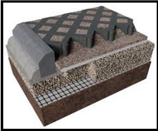
Fig 5.2 Pervious unit paving
